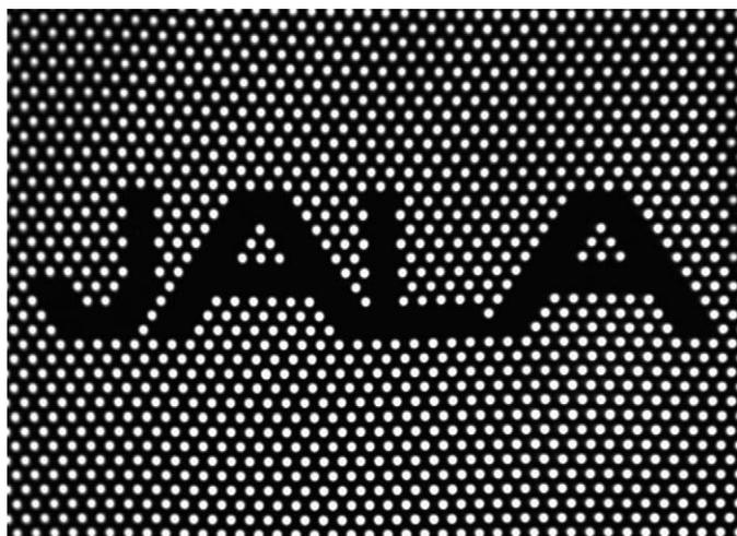
**Figure 7.** Selected 200- $\mu\text{m}$  diameter wells are aspirated from a portion of a 100,000-well GigaMatrix plate filled with 1  $\mu\text{M}$  fluorescein to demonstrate precision recovery.
