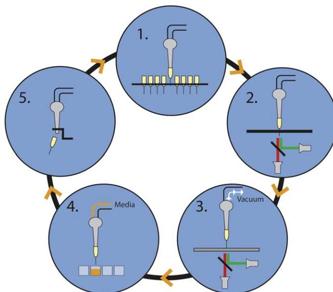
**Figure 5.** Basic steps of the hit recovery process: (1) Mount and locate the tip of a sterile recovery needle; (2) align the recovery needle to the well containing the putative hit; (3) aspirate the contents of the well into needle; (4) dispense the needle contents into microplate well; and (5) remove and dispose of the used needle.
