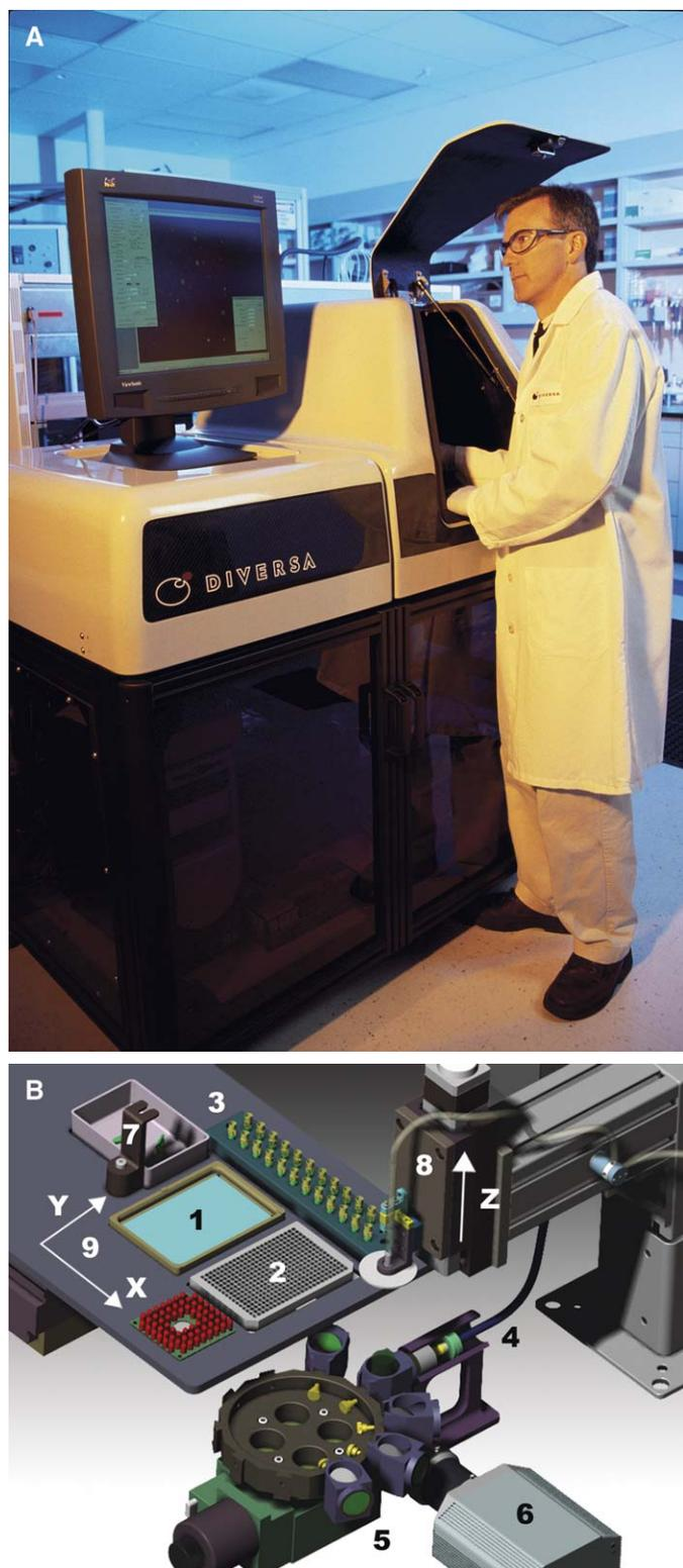
**Figure 6.** (A) Automated detection and recovery system and (B) exploded 3D model view of the major detection and recovery station components. (1) GigaMatrix plate, (2) recovery microplate, (3) recovery needles, (4) illumination optics, (5) filter wheel, (6) cooled CCD camera with telecentric lens, (7) needle removal device, (8) needle axis translation stage, and (9) XY translation deck.
