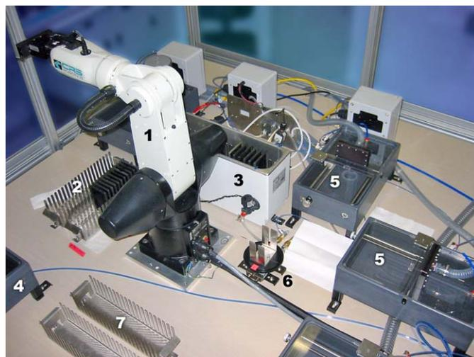
**Figure 8.** Automated GigaMatrix plate cleaning system. (1) Articulated robot arm, (2) input plate rack, (3) ultra sonic cleaning bath, (4) fluid removal stations, (5) fluid flushing stations, (6) regrip station, and (7) output plate rack.
