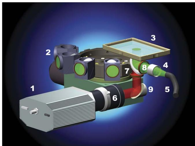
**Figure 4.** A 3D model of the detection system. (1) Cooled CCD camera, (2) filter wheel, (3) GigaMatrix plate, (4) excitation focusing lens, (5) fluid filled light guide, (6) telecentric lens, (7) fluorescence emission filter, and (8) fluorescence excitation filter.
